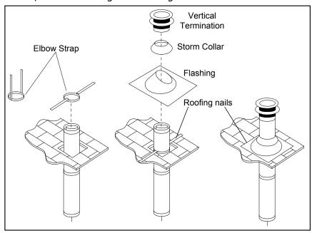
Figure 28. Vertical Vent Termination
